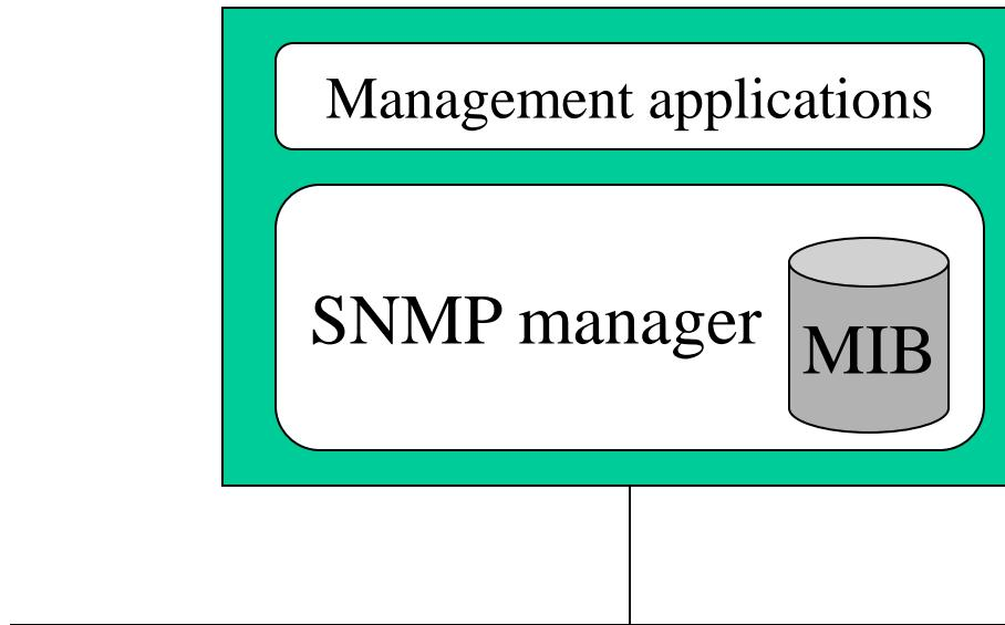
**SNMP defines how to get and change data in MIB of a host/device**
